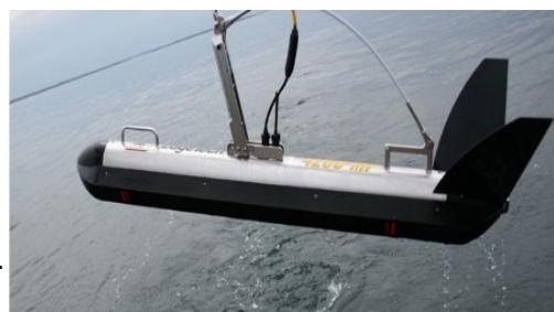
The SSS will be dual frequency hydrographic sonar with the lowest operating frequency of 300 to 900 kHz but not less than 100 kHz.
